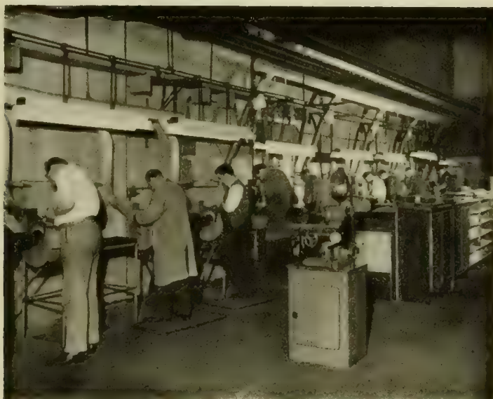
Fig. 4. Surgical instrument grinding and polishing
